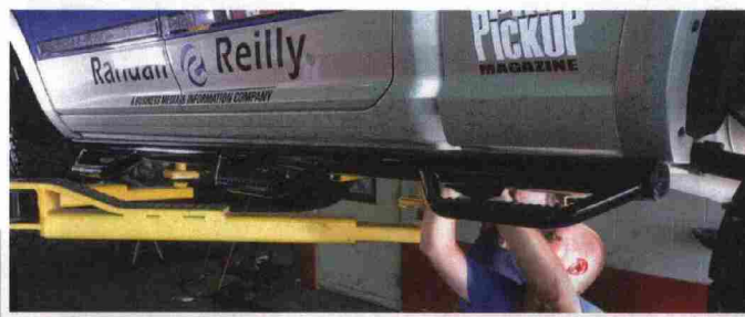
N-Fab nerf steps add an extra layer of body protection to the Big Boss' rockers, while giving us a leg up getting in.
