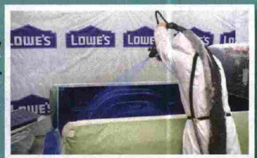
Line-X sprayed the bed and rockers with their new Xtra coating material, which is color-matched to our Ram.
