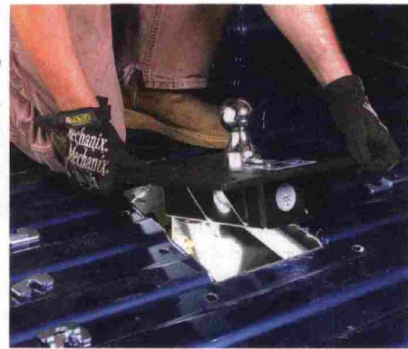
A fold-down gooseneck hitch from Curt Manufacturing is fitted into the bed prior to being sprayed with Line-X.
