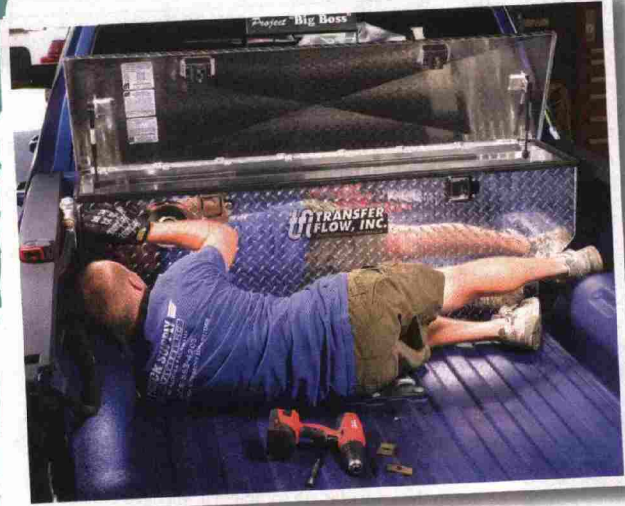
Ben Allen installs the 30-gallon Transfer Flow crossbed refuel tank/tool box at the TSO shop.
