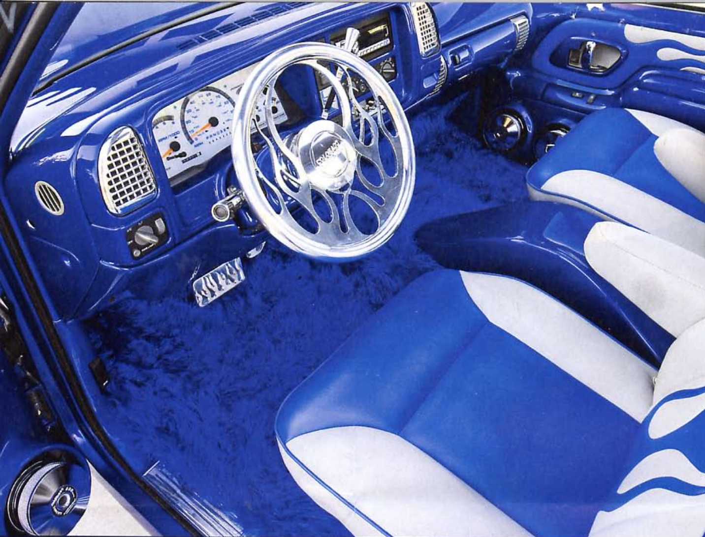
Inside the shaved doors, the dash was painted to match, the seats recovered in Enduratex vinyl, and every Empire Motorsports billet accessory was added.
