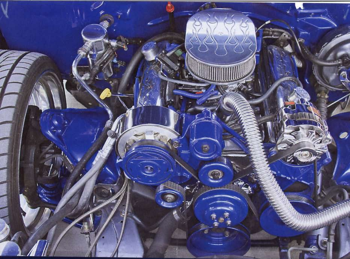
Tricks, like having the frame and suspension painted along with polished hard brake lines and billet accessories, really make an engine compartment stand out.
